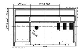
**5mm safety around display** for static elements to deal minor changes in dimensions and avoid any mechanical stress
