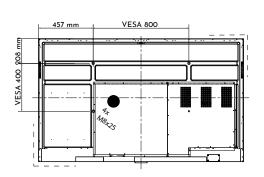
**5mm safety around display** for static elements to deal minor changes in dimensions and avoid any mechanical stress
