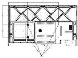
**5mm safety around display** for static elements to deal minor changes in dimensions and avoid any mechanical stress
