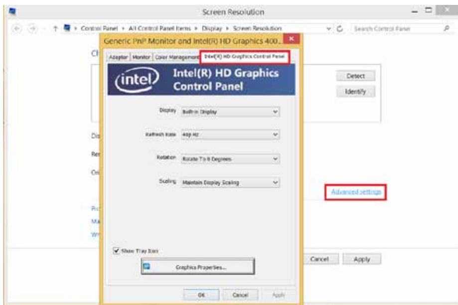
Click “display” and select the screen that needs to be scaled. Either your computer display (for laptops called “built-in display”) or the monitor/projector. Click “scaling” and choose “scale full screen”. Then click “apply”. If necessary, have both scaled to full screen.
