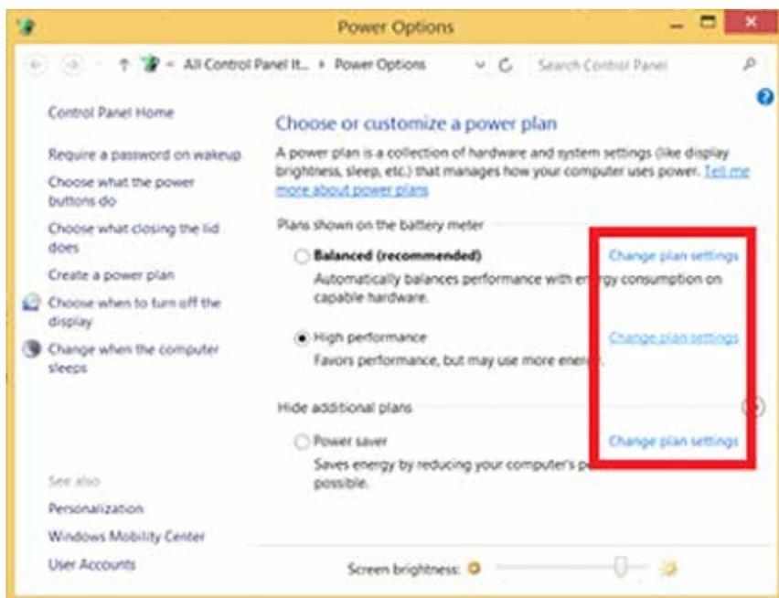
For each power plan used (!) click USB Settings -> USB selective suspend settings -> disable both “On Battery” and “Plugged In”
