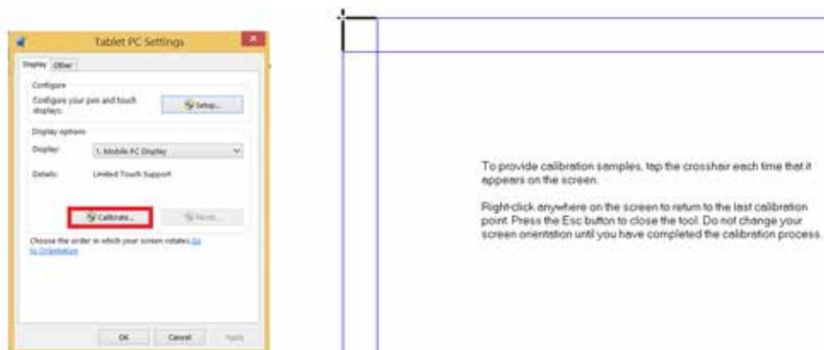
After having pressed on all the black crosses, the calibration is finished and the calibration should be fully accurate. If this is still not the case, contact your i3DEALER. Keep in mind the windows calibration tool only enables 7 touch points (windows 7 and higher).
