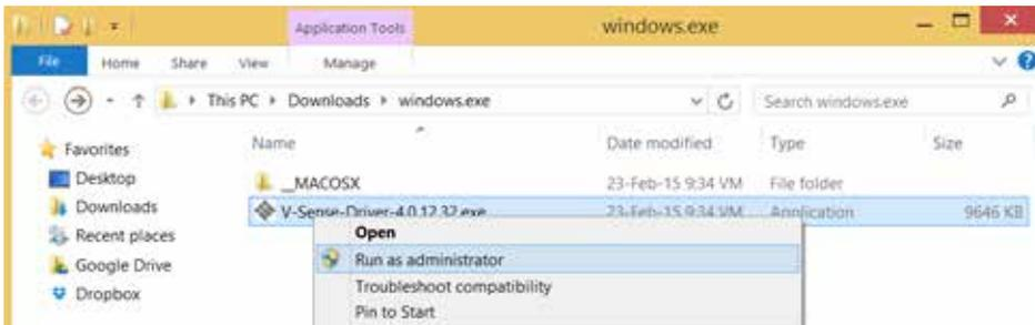
Run the installer and click 4 times “next” and finally “install”. If you can finish the installation, the drivers will ask for a reboot. Reboot your computer to finish the installation.
