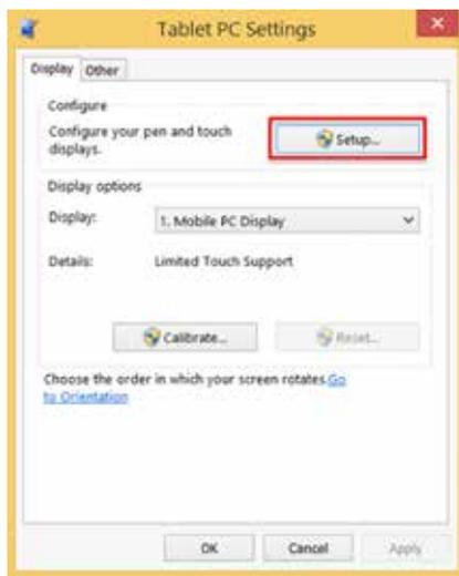
Follow the on-screen instructions. Tap on the board when the below instructions are shown on the board or press "enter" when you read the instructions on your computer screen only. With this step you identify the board as the touch screen to be used in windows. Finish with "escape".
