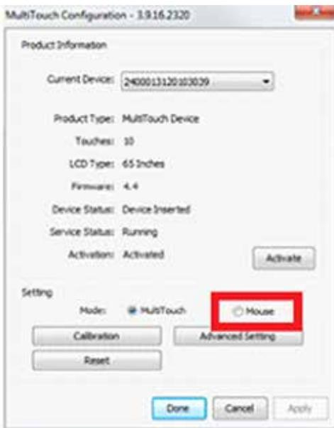
if you don't have touch using "mouse" mode, check your system settings (Control Panel\All Control Panel Items\System). If the drivers are working the pen & touch should indicate 32 touch points.
